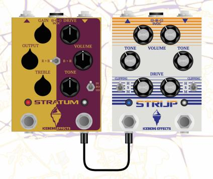
When leaving the Stratum pedal in its default settings and connecting it to another Iceberg effects pedal (the Strijp in this example), pressing the connected footswitch (footswitch A of the Stratum and footswitch B of the Strijp in this example), will either toggle between the two effects or
