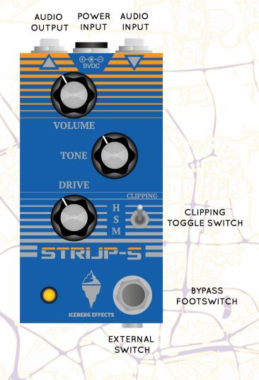
Audio Input Connect the Strijp-S pedal to your guitar or another effect pedal using a 6.35mm (1/4") mono TS audio cable.
