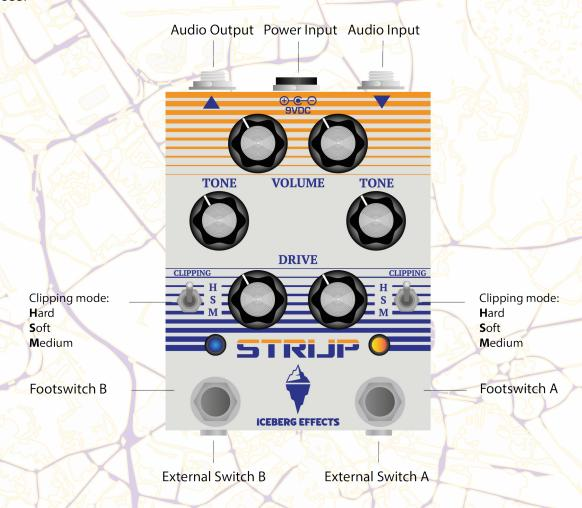
Audio Input Connect the Strijp pedal to your guitar or another effect pedal using a 6.35mm (1/4") mono TS audio cable.
