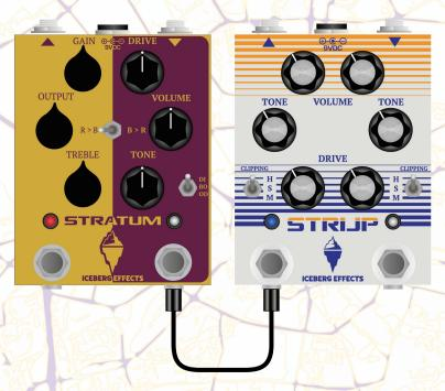
When leaving the Strijp pedal in its default settings and connecting it to another Iceberg effects pedal (the Stratum in this example), pressing the connected footswitch (footswitch A of the Stratum and footswitch B of the Strijp in this example), will either toggle between the two effects or engage/disengage both pedals at the same time, depending on the footswitch state before connecting the pedals together.
