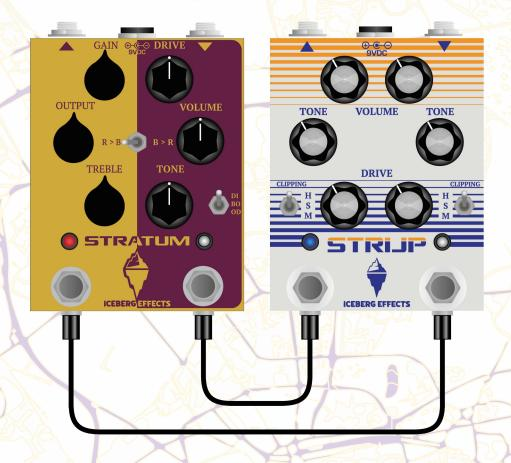
You want to take the toggling experience one step further? Why not use two 3.5mm cables and connect both sides of the pedals? When leaving the bypass mode and external bypass modes in default (Normal and Toggle, respectively), pressing any of the connected footswitches will toggle between those effects.
