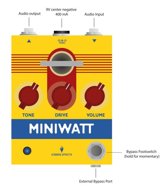
**TONE** - Works as a tilt EQ control. Turn it past noon to boost treble frequencies and cut bass frequencies. Turn it below noon to amplify bass and attenuate treble.
